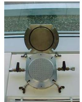
Test Cell for Phase 1 of the Gas Permeability Research Project
