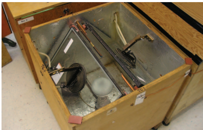
The volatile fogging box is one of the tests for IG certification.
