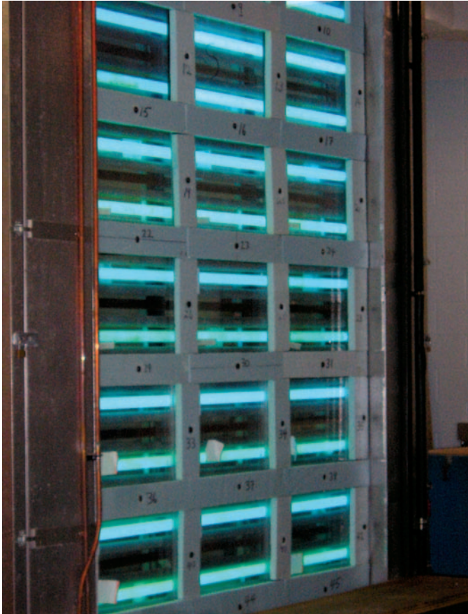
In accordance with ASTM E2190, IG units must undergo weather cycling in a testing chamber.
